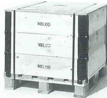
Wooden case for coils (in horizontal position) Z100 Coils with interleaving cardboard Frame with cover. Height: max. 70 cm (27.5 inch), Weight: max. 800 kg (1770 lbs)
